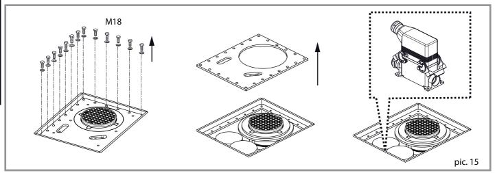
A watertight box is factory-fitted inside the bollard and pre-wired with all the required electrical connections to the bollard (electric motor, limit switches, LED lights).
