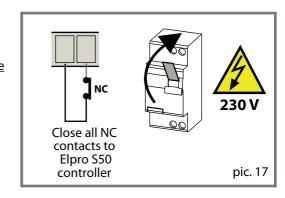
[c] Check the electrical connections to the limit switches. Once the system has been power supplied, check the LEDs status first of all: with the post in the lowered position L12 LED is OFF, while L13 LED is ON. If this does not happen, swap connections to terminals 11 and 12 on the Elpro S50 control board.
