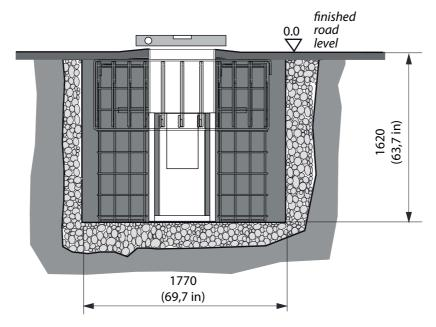
Concrete casting: let it set firmly for 7 days before carry on with the installation of the bollard
