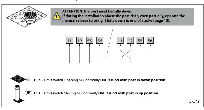
B) Once electric power is supplied, provided that the LEDs of the limit switches are correctly alight (post down L12 led OFF), by the first pulse the post should rise. If not, swap the connections to the motor live terminals (on Elpro S50) after having disconnected the electric power supply from the installation.
